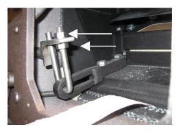
When properly adjusted, you should have to apply some pressure to the bypass lever to close the cover completely.
