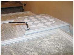
2. Treat all hardware to be removed with penetrating liquid. Allow it to stand at least 15 minutes. Use a <sup>1</sup>/<sub>2</sub>" wrench to remove the nuts that attach the u-bolt to the bypass shaft and lift guide. Remove the u-bolt. Pay attention to the direction the u-bolt was installed.
