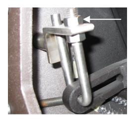
Remove the (2) bolts that attach the lift guide to the bypass cover with a 1/2" socket.
