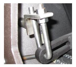
5. Test the seal between the bypass cover and the gasket using a slip of paper. Close the bypass cover on the paper. There should be enough resistance on the paper to slightly curl it when it is pulled out. To increase pressure on the bypass door, loosen the top nut on the U-bolt, and then turn the bottom nut counter clockwise. To decrease pressure on the bypass door turn the bottom nut clockwise, and do the same to the top nut. Make small adjustments until the proper seal is reached.
